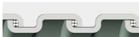
Square-Locked Design with cord packing 3/8" through 1-1/4"
